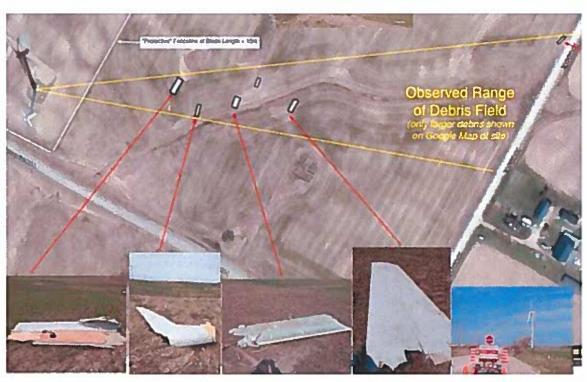
Debris at 150m from tower -1.3m X 3.6m Debris at 170m from tower Debris at 210 m from tower 1.2m X 3.0m
