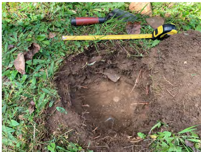
Plate 14: Test Pit 3- Showing stratigraphy typical of the eastern Study Area edge. Medium brown silty loam topsoil with heavy pebble and cobble inclusions (Lot 1) over yellow-buff sand subsoil with pebble inclusions (Lot 2) (Photo 4774).
