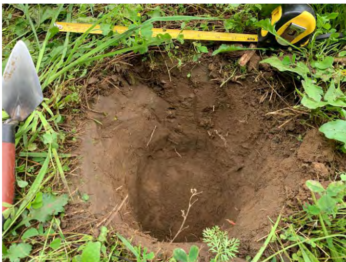
Plate 11: Test Pit 2- Showing typical stratigraphy across the western end of the Study Area. Medium brown silty loam ploughzone (Lot 1) over orange brown silty sand subsoil (Lot 2) (Photo 4772).
